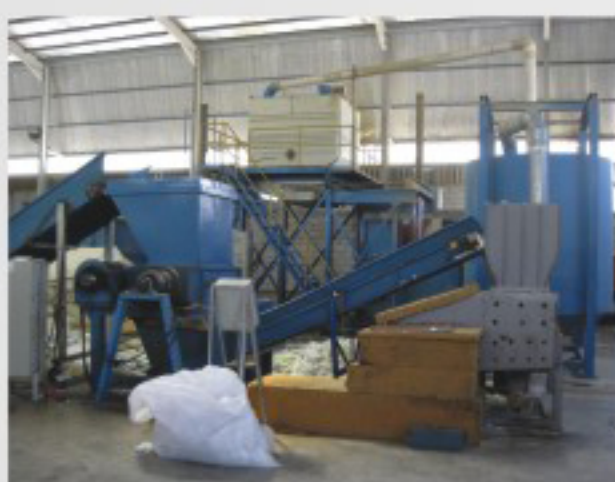
Complete Image of Re-Bounding Foam Making System
